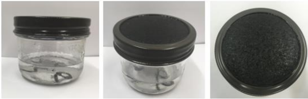
Figure 3.2 An example of a sample container. The same sample container set up is used for wet cup and inverted wet cup vapour permeance testing.
